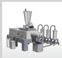
④ Weighing/Kneading The positive and negative electrode materials are measured out in suitable amounts and mixed into pastes.
