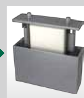
⑰ Cell case insertion The wound body is inserted into the cell case.
