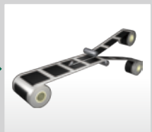
⑥ Slitting The rolls of electrode material and separator are cut into the appropriate size.
