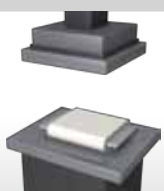
⑮ Press The wound up element is pressed.
