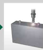
⑳ Pouring plug welding The pouring plug is welded and the battery cell is completely sealed.
