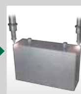
⑱ Cell lid welding The cell case and lid are laser-welded.
